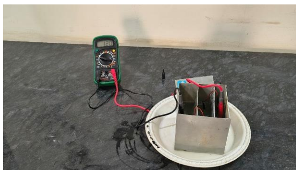
Fig. 2. Complete experimental setup demonstrating the electrodes immersed in the Aloe Vera gel matrix connected to a digital multimeter.
