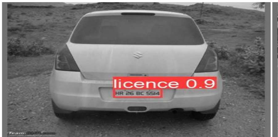
Fig 4. Shows the fetched result of number plate after detection using paddle OCR.
