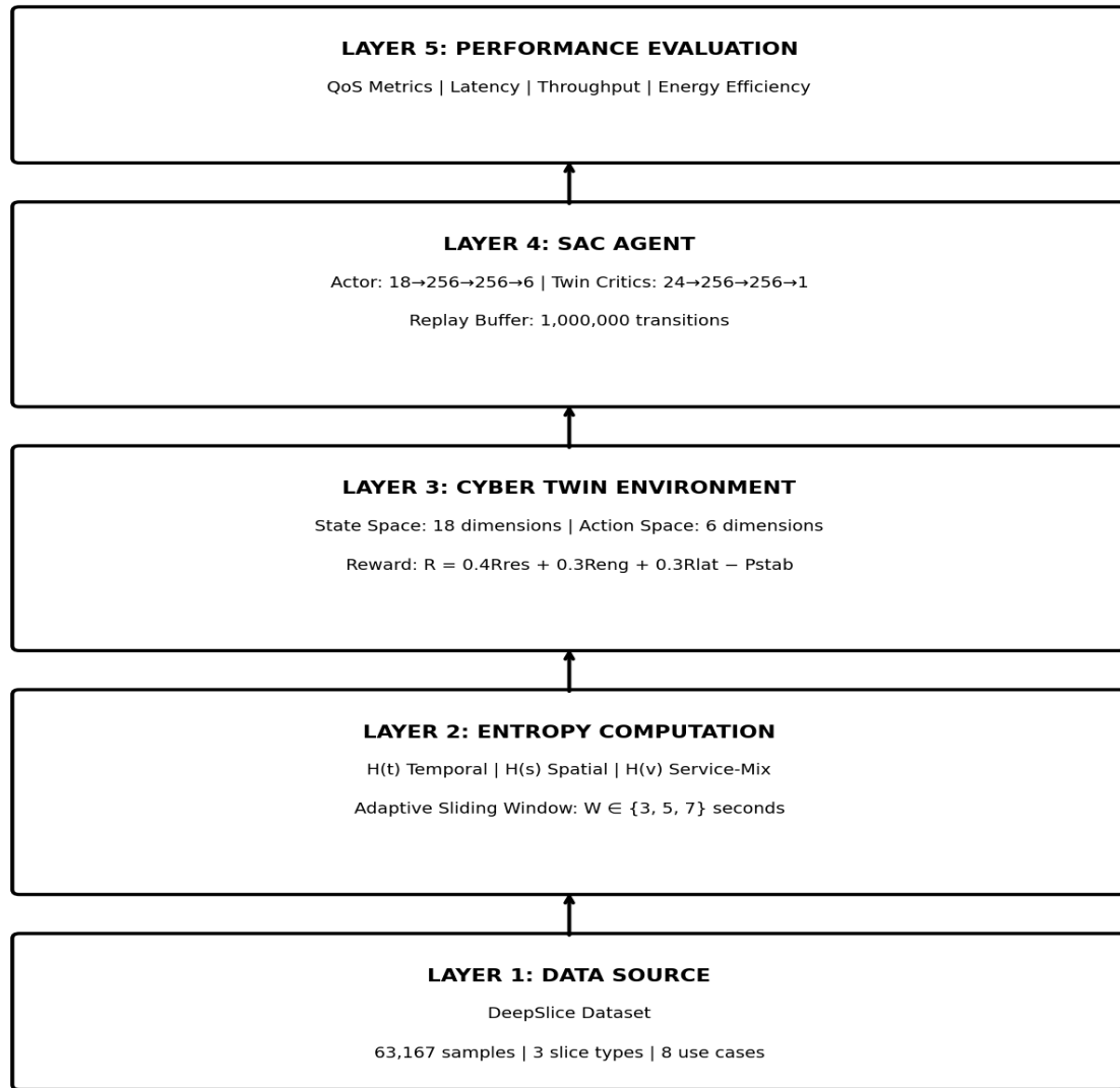
Figure 1: Five-Layer Framework Architecture for Cyber Twin-Driven Resource Allocation.
