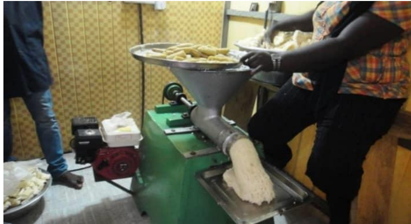
Figure 6: Modified Cassava Fufu/Yam Pounding Machine
