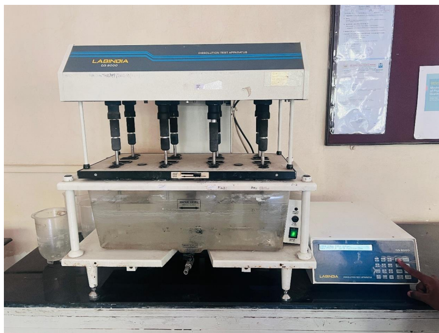
Figure c Dissolution Test Apparatus.
